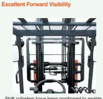
Shift cylinders have been positioned to enable clear forward visibility.
