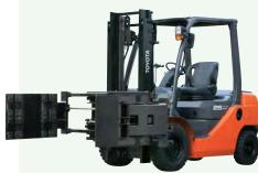
Applications Can clamp from one, two or four drums at a time. Its side shift function provides effective utilization of limited storage space.
