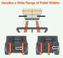
Forks are moved hydraulically to match the width of the pallet. No need for the operator to leave the forklift to adjust fork width.
