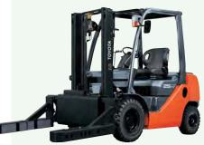
Applications Allows blocks to be handled smoothly and precisely without a pallet. Its side shift function provides effective utilization of limited storage space.
