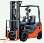
Applications Recommended for locations that have a variety of pallet widths. Its side shift function provides effective utilization of limited storage space.
