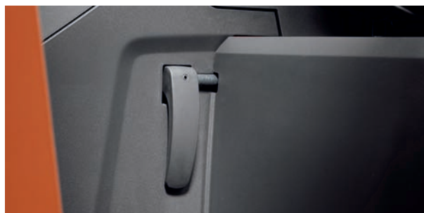
The battery is manually released with a lever on the battery wall enabling easy battery change without the operator needing to dismount
