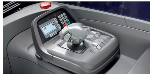
An optional multifunction control unit can be selected, depending on the preference and experience of your drivers
