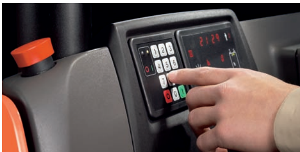
Unique to BT, N-series offers PIN-code entry as standard to ensure that the truck is only used by authorised personnel
