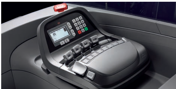
Standard mini-levers allow fingertip control of each fork movement
