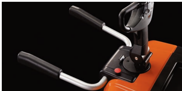
Folding sideguards offer protection to the operator without compromising the manoeuvrability advantages of the flip-down platform
