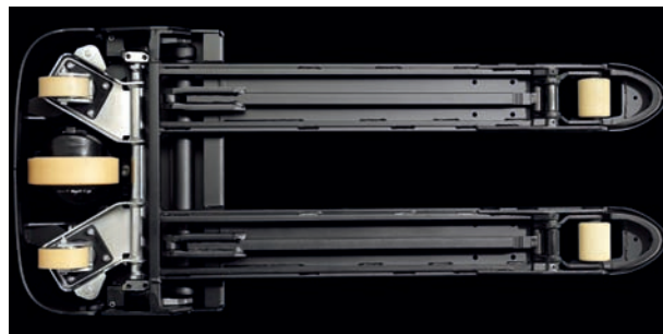
BT's unique 5-wheel chassis improves stability on ramps
