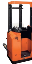
S-series 1350 kg–1600 kg Max. lift height: 6,3 m
