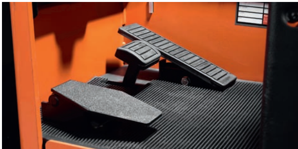
Pedal layout is as in a car, optimising safety and productivity
