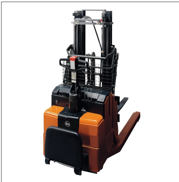
The RWE120 is a pedestrian reach truck with moving mast. It also has adjustable width forks, for mixed or bottom-boarded pallet handling. Its maximum lift height is 4.8 m and load capacity 1200 kg.
