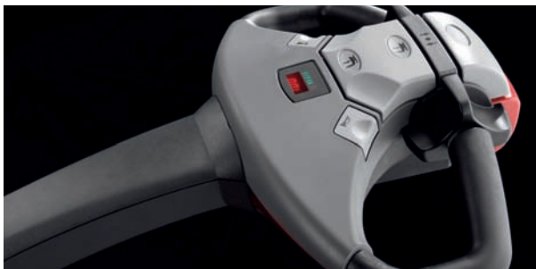
The tiller arm's control handle incorporates BT Powerdrive technology, for easy, intuitive control
